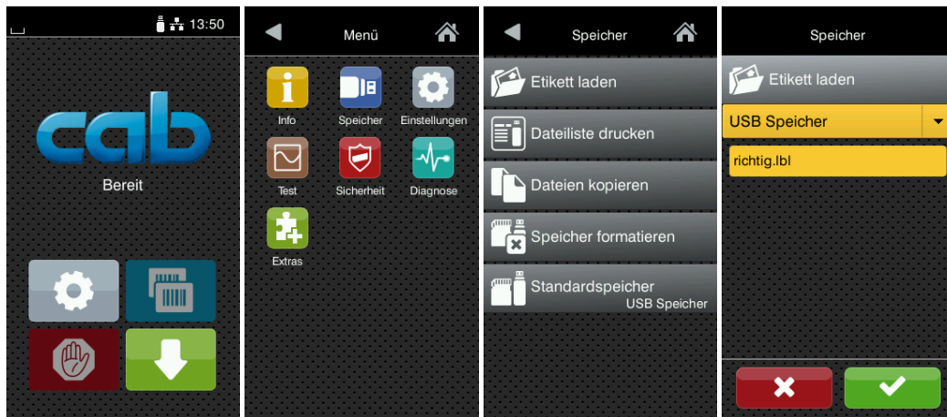
Figure 2.1: Via the gray gear wheel symbol and the blue memory stick button you get to the menu “Storage”. Here you can see the data stored in the subfolder “labels” to load copied JScript label files.
