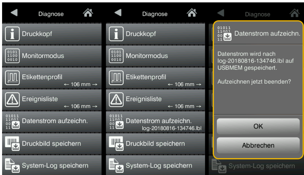
Figure 10.2: A SQUIX printer allows to record all incoming data into a file directly on an USB storage device
