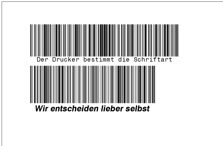
Figure 4.16: The upper barcode has a plain text line generated by the printer, the lower barcode has its own formatting. The field name SELFMADE ensures that the correct content is always printed under the barcode if you change it later with only one R command. (Created by listing 4.13.)
